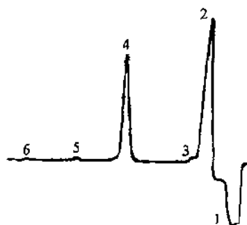
Fig. 6 GC chromatogram of the products obtained from the equilibrium polymerization of D_4 Eluting peaks: (1) ethanol, (2) toluene, (3) D_3 , (4) D_4 , (5) D_5 and (6) D_6
